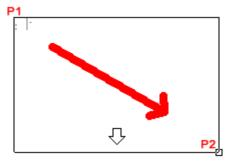
Start the Multiline Text command, and pick a spot in the drawing. Drag the cursor over to create a 'rectangle' to represent the area you want your text in, and pick the other corner. As soon as you pick the second point (P2), the full Multiline text editor will appear. Type your text, and press OK when done.
