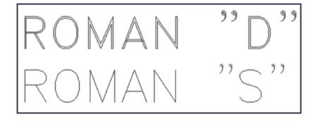
In later versions of AutoCAD, there is an easy way to change existing text to a new style. First, select the text, then go up to the Text Style Menu (usually towards the top of the screen) and select the style you want from the droplist (below) and the text will change automatically.
