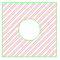
Note that AutoCAD recognized the circle in the middle and didn't hatch over it. If the lines appear 'jagged', don't worry - it is a video display issue -the prints will come out clean and straight.
