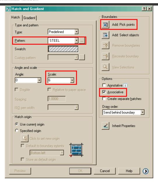
As usual, start at the top of the dialog box and work your way down. We're going to say that this is a cross section of piece of steel, so choose the predefined Hatch pattern called **STEEL**.
